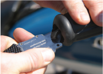
3. We started the installation by using a knife to cut out the end of the rubber grip.
