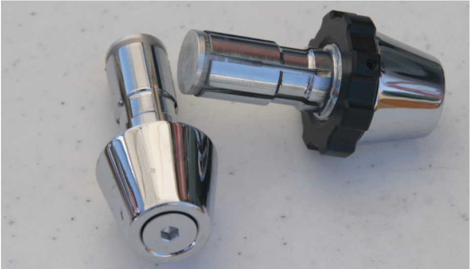
1. For this installation we opted for the chrome Torpedo (MSRP $195.00) E-Z Cruise Control. The kit comes with two Torpedos, the throttle side (right) and a matching unit for the left side.
