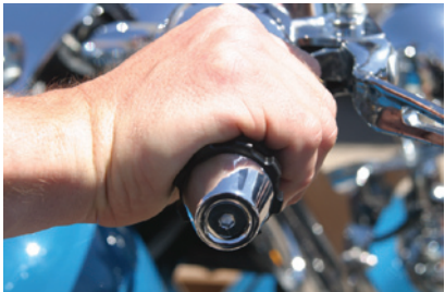
7. When it came to using the E-Z Cruise Control all we needed to do was grip the friction nut (serrated portion) between our pinky finger and palm and rotate it so that it pinched or "locked" the throttle in place. Then we rotated the friction nut in the opposite direction to relieve the throttle. When in the locked position, the friction nut is set up so that you can still open and close the throttle as needed, it's just a little stiffer. A simple solution for much needed relaxation.
