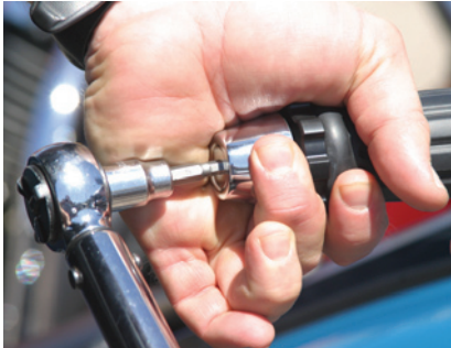
4. Then the Torpedo for the throttle side was slid into the grip end and torqued to spec.
