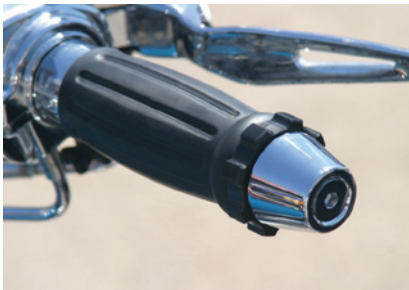
4. Then the Torpedo for the throttle side was slid into the grip end and torqued to spec.
